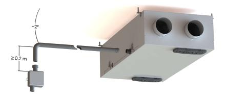
Figure 7. Connecting the condensate drain
