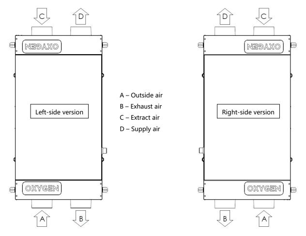
Figure 2. Mounting orientation
