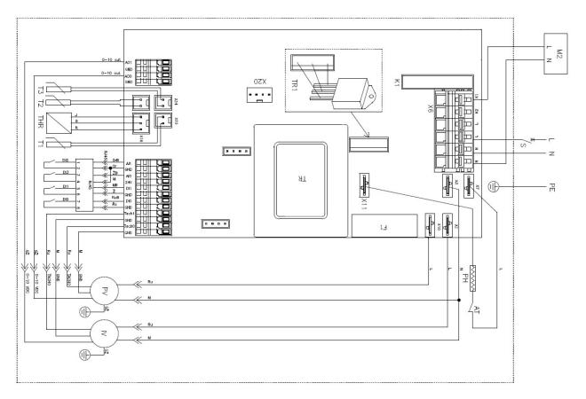
Figure 12. Control board electrical wiring diagram
