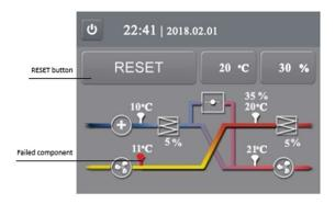
Figure 27. Failure indication
