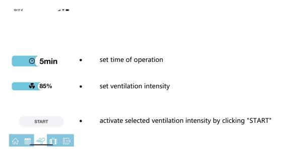
Figure 19. Ventilation boost activation
