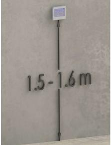
Figure 9. Installation of the control panel
